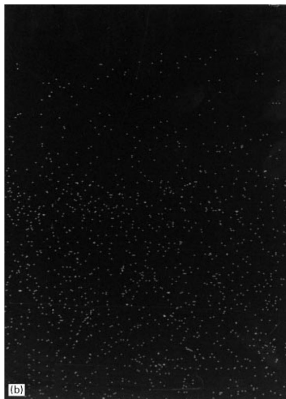
Figure 5 Cross-section SEI of the Bondex cement after contact with 0.01 M citric acid for 1 wk: (a) SEI, (b) ZnK \alpha imaging.
